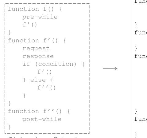
Take the synchronous (Design pattern 16) and apply Rules #1 and #2 to get the asynchronous (Design pattern 17)
