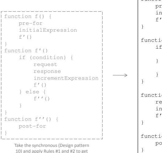
the asynchronous (Design pattern 11)
